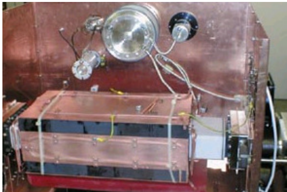
The ferrite-core water-cooled RF-dipole with a transverse RF magnetic-field integral of 1.5 Tmm peak-to-peak.
